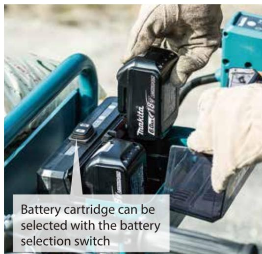
Battery cartridge can be selected with the battery selection switch
